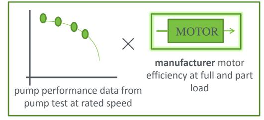
Manufacturer can pair its pump data with manufacturer motor data tested in accordance with DOE motor TP.
